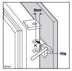
Remove the squares and mark a distance of 8 mm from the outer edge of the door where the nail must be fitted (K).
